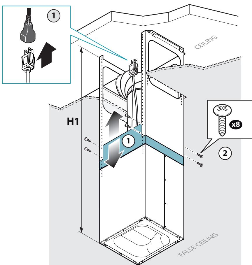
**EN** - Low ceiling installation. Securing of the bottom trestle and the motor chamber to the ceiling(10) NRS pipe installation (11).
