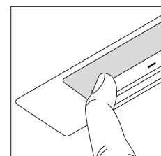
⚠ If the pushbutton panel is completely inactive, before contacting the Technical assistance service, disconnect power temporarily to the appliance (about 5''), possibly by acting on the main switch, to restore normal operation.
