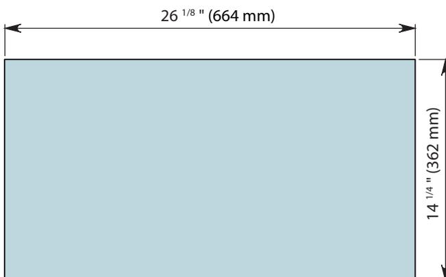
EN - HOLE MEASUREMENTS FOR INSTALLATION
